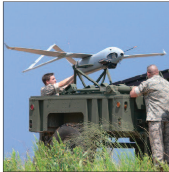
Entire Launch and Recovery Trailer (LRT) deployed in one HMT
