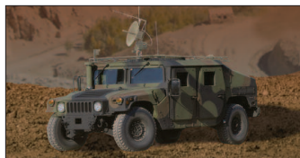
EGCS deployed in an on-the-move command and control configuration
