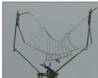
Aerosonde demonstrating shipboard Soft Hands® recovery
