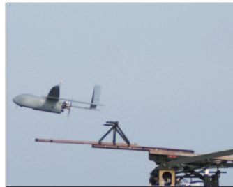
Aerosonde® conducting shipboard flight operations and launch
