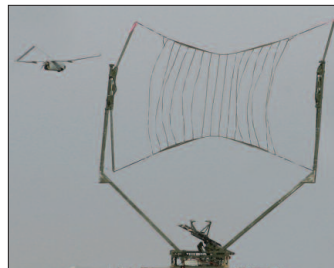
Aerosonde conducting shipboard flight operations, making a precision approach
