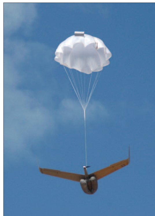
An automatic parachute and air bag recovery system can be deployed virtually anywhere.
