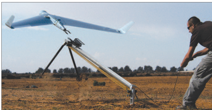
The Orbiter Mini-UAS launches using a catapult that incorporates redundant safety features.
